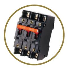
Mounting - These circuit protectors are designed to mount on standard 35mm DIN rails, such as 35x7.5 or 35x15 per DIN EN50022. Other specialty rails are available from suppliers that provide a means of mounting non DIN mount components by means of special captive jam nuts.
