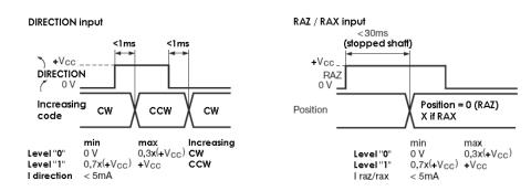
Note: Do not connect other pinouts, connect DIRECTION and RAZ to a potential (RAZ at OV if not used).
