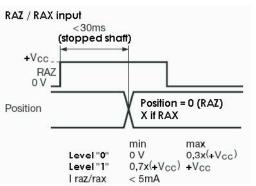
Nota : Do not connect other pinouts, connect DIRECTION and RAZ to a potential (RAZ at 0V if not used)
