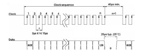
**Transmission:** Transmission up to 400m at 100kHz in function of the cable characteristics.
