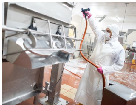
This cleaning process goes smoother when the operator has access to all parts of the equipment.
