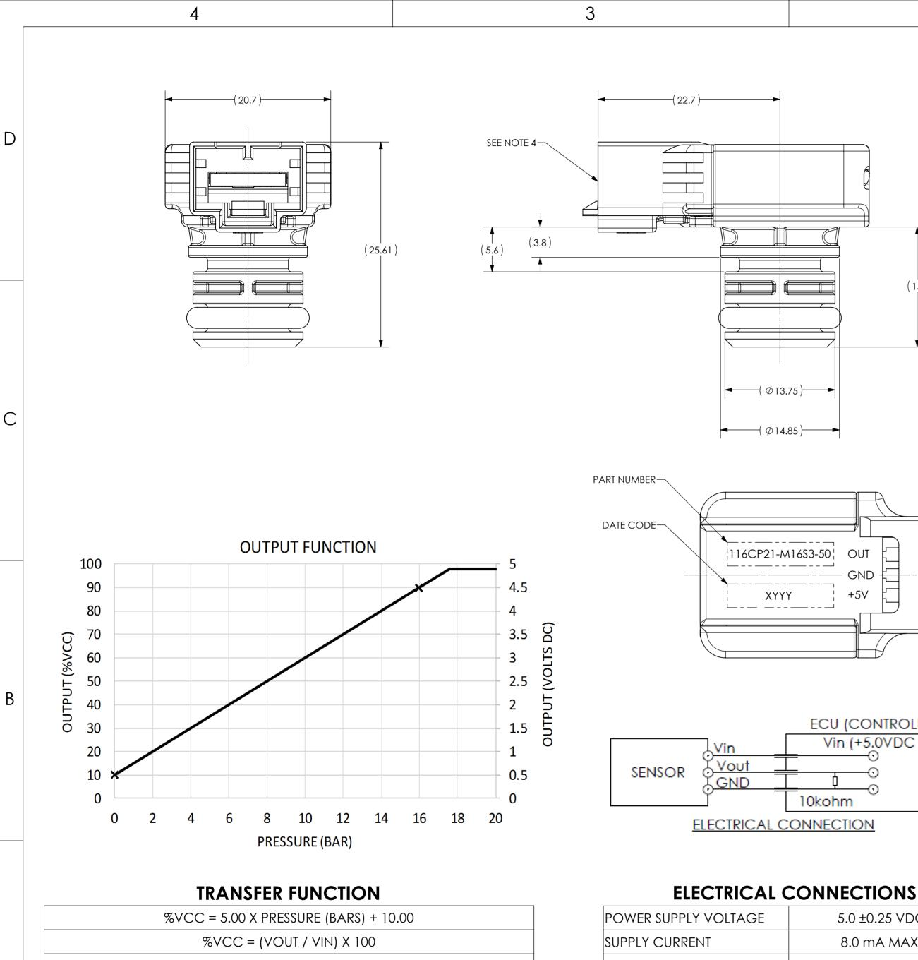
PRESSURE (BARS) =  $20.00 \times (VOUT/VIN) - 2.00$ FOR REFERENCE ONLY (VIN = 5.0V), PRESSURE (BARS) = 4.00 X VOUT - 2.00
