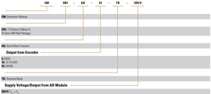
**28V/5:** V<sub>out</sub> = 5 VDC **28V/0C:** V<sub>out</sub> = 0pen Collector
