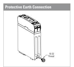
Protective Earth (PE) screw type recommended is 10-32 UNC standard not provided with SSR. Through the use of a DIN rail ground (protective conductor) terminal block, the DIN rail itself can be used as the grounding bus bar. In this case, the zinc plated steel material used for the DIN rail clip of DR22 models, permits a secure path to ground and avoid the need of a further PE connection.
