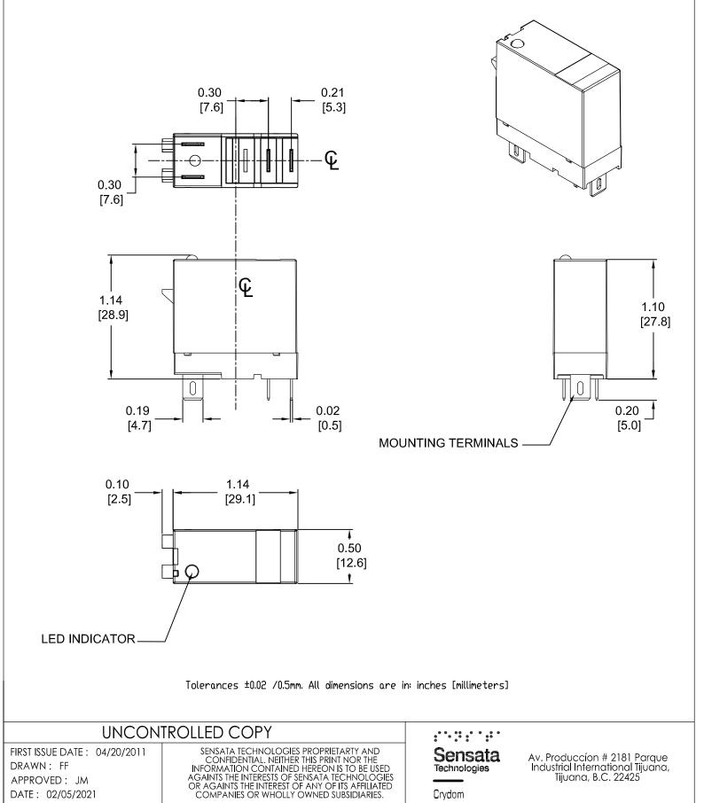
DATE: 02/05/2021 Crydom TITLE UNLESS OTHERWISE SPECIFIED DIMENSIONS ARE IN INCHES [MILLIMETERS] AND ARE INTENDED AS NOMINAL. SEE PRODUCT SPECIFICATION FOR MORE DETAILS. **ED SERIES SMALL** ECN: DWG NO. REV. SIZE 108802 DO NOT THIRD ANGLE DATE: **SCALE PROJECTION SOLIDWORKS SCALE** N/A SHEET 1 OF 1 DRAWING
