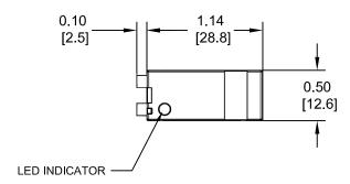
Tolerances ±0.02 /0.5mm. All dimensions are in: inches [millimeters]
