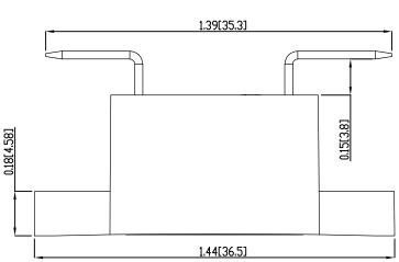
Tolerances ±0.02 /0.5mm. All dimensions are in: inches [millimeters]
