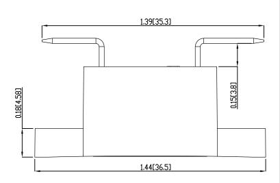
Tolerances ±0.02 /0.5mm. All dimensions are in: inches [millimeters]
