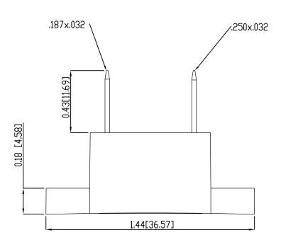
Tolerances ±0.02 /0.5mm. All dimensions are in: inches [millimeters]
