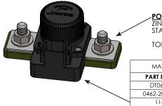
POWER CONNECTION ZINC PLATED STEEL, M12X1.75 BOLT STAINLESS M12X1.75 FLANGED NUT
