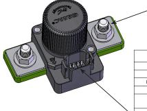
POWER CONNECTION ZINC PLATED, M12X1.75 BOLT STAINLESS M12X1.75 FLANGED NUT
