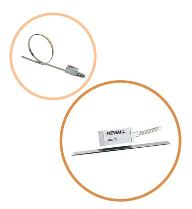
Newall<sup>®</sup>'s MAG-TS encoder consists of a reading head that travels along a magnetically encoded tape. The tape is made of a ferrous backing affixed to a flexible magnetized rubber substrate that is protected by a stainless steel cover strip.
