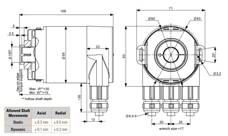
Shaft diameter can be reduced to 12mm, 10mm or 8mm by reduction ring (by inserting them into the hollow shaft)
