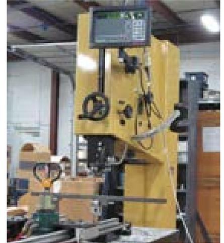
When Multi-Wing implemented this process almost 20 years ago, they originally settled on the use of glass scales. Initially, they experienced problems with scale contamination, due to fiberglass/aluminum dust, which ultimately led to scale damage. Once they discovered Newall, they quickly determined that this was the ideal solution to eliminate their contamination issues, scale damage and meet their accuracy requirements.
