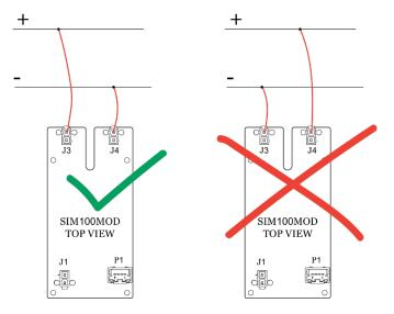
Figure 5: Proper connection to IT power system terminals
