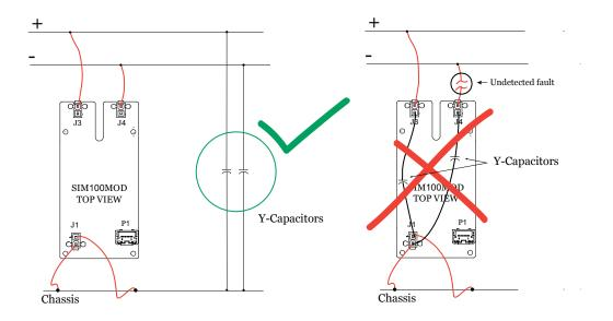
Figure 7: Presence of Y-capacitors is a requirement for proper function of the SIM100MOD. The capacitors should be connected directly to the power lines. Connecting them on the SIM100MOD board instead would impair the ability of the monitor to detect disconnection from the monitored IT power lines.
