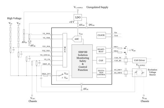
Figure 1: SIM100MOD functional diagram
