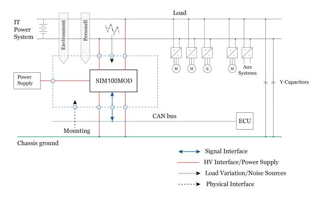
Figure 2: The boundary diagram of SIM100MOD as SEooC in EV implementations
