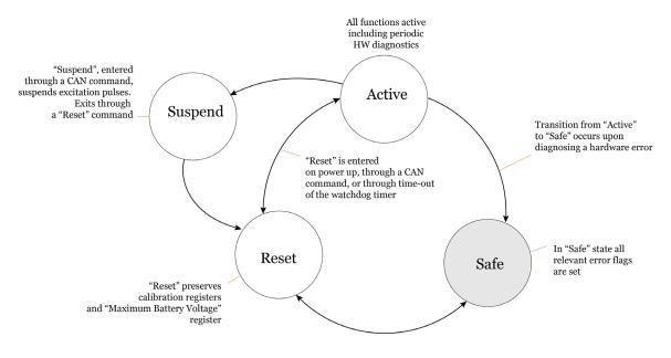
Figure 4: Operating states of the SIM100MOD
