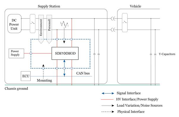
Figure 3: The boundary diagram of SIM100MOD as SEooC in EV implementations
