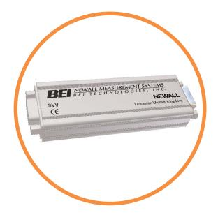
The SVV/SVM Sine-Cosine converters takes the quadrature, differential, output signals from a suitably matched DSG-EV/EM or DMG-EV/EM encoder and converts these signals to analogue Sine and Cosine levels.
