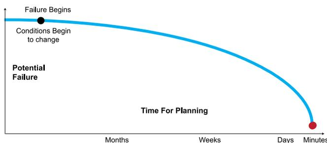
P-F Curve, indicating the time interval between a potential failure and a functional failure; the P-F Interval.
