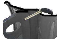
Torque screw to complete installation
