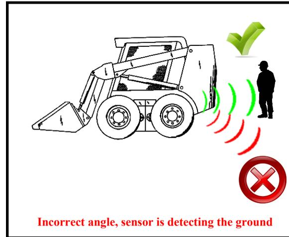
The Sensor should be centered on the rear of the vehicle for best coverage. **Caution:** The tilt angle of the sensor will determine the path of the radar. (See image above)
