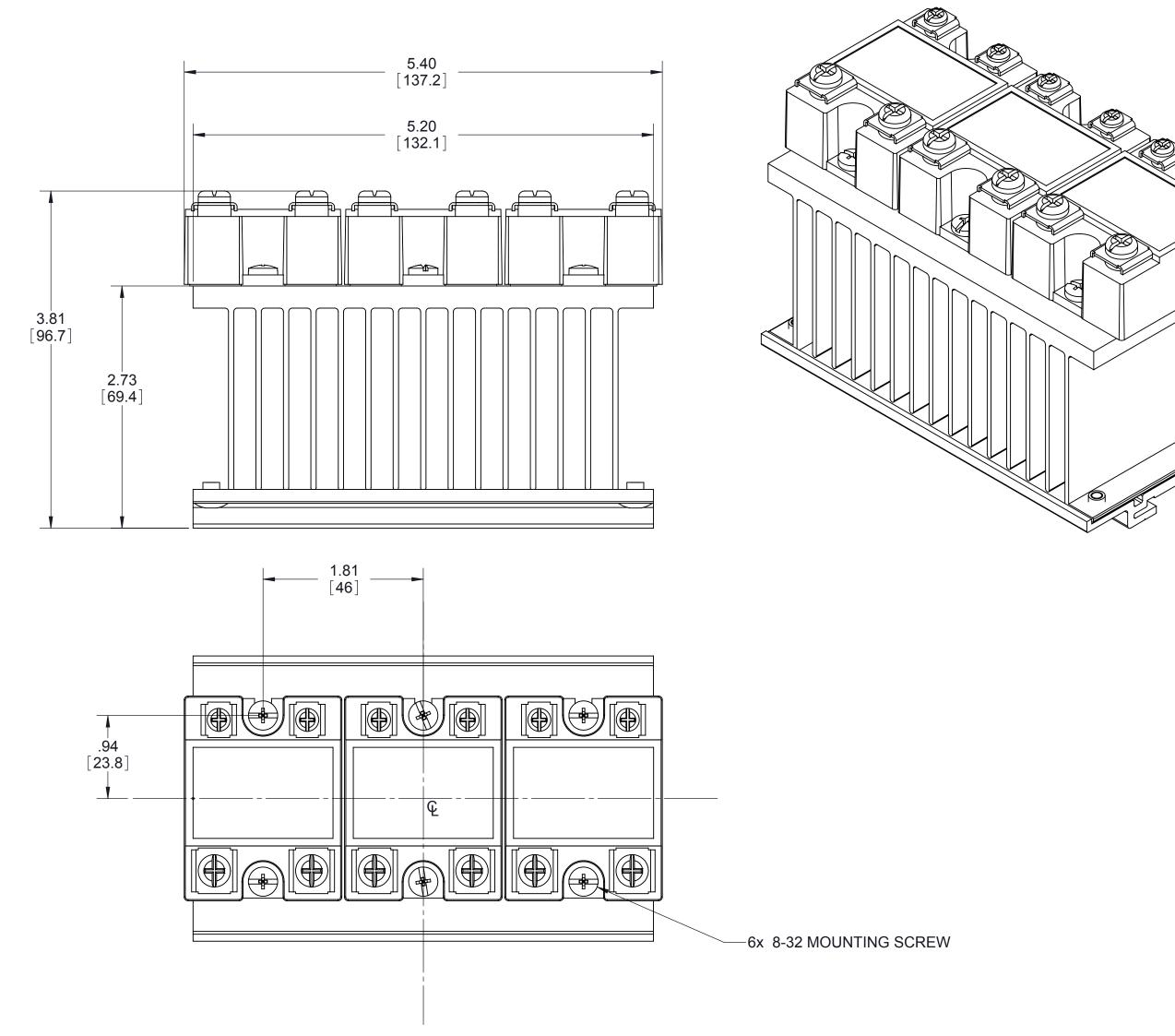
Tolerances: ± 0.02 in / 0.5 mm. All dimensions are in: inches [millimeters]
