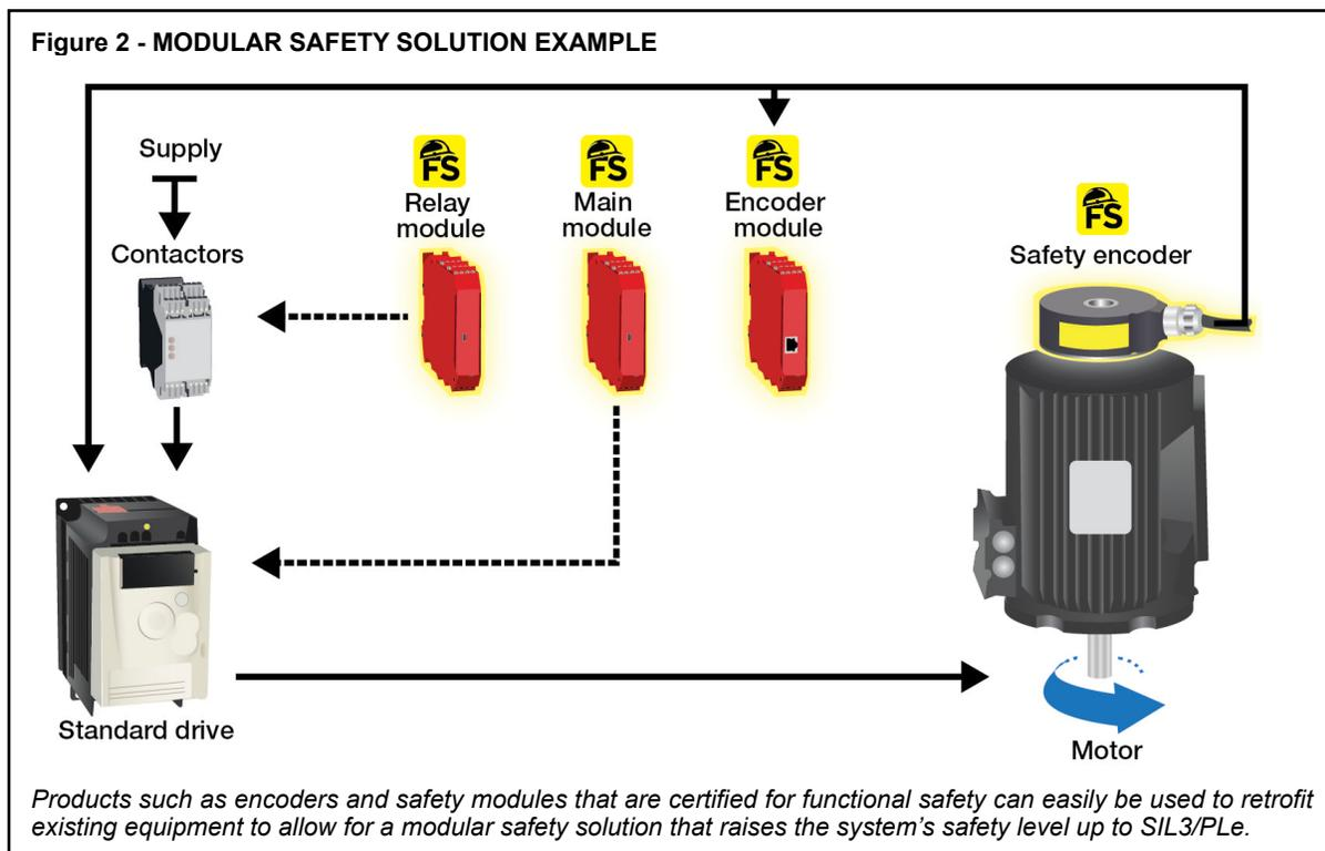
refurbishing/upgrading existing systems. Engineers can simply swap out older components for new, and in doing so immediately improve a system's overall Functional Safety level. These newer components are often more sophisticated and a single device can sometimes be used to perform tasks that previously may have required multiple devices to achieve the same level of safety.
