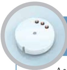
Packaging is very simple, by clamping the ceramic transducer in a metal can and using an elastomere seal for medium pressures. This principle is commonly accepted as the most cost effective pressure sensing technology for pressure ranges between 1 and 100 bar.
